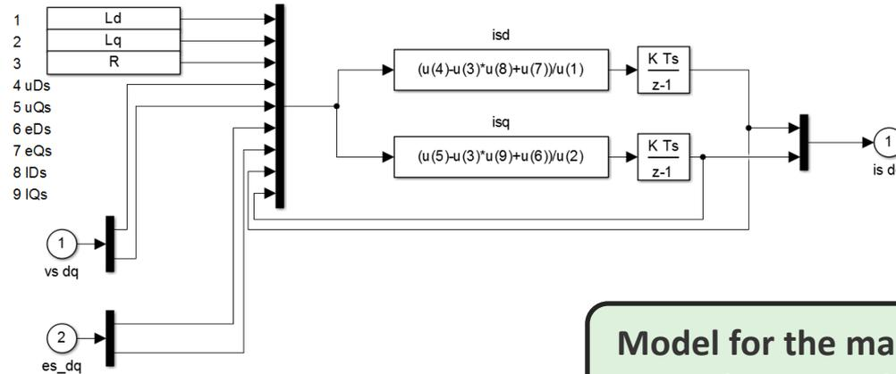
Model for the machine windings and the electromechanical conversion
