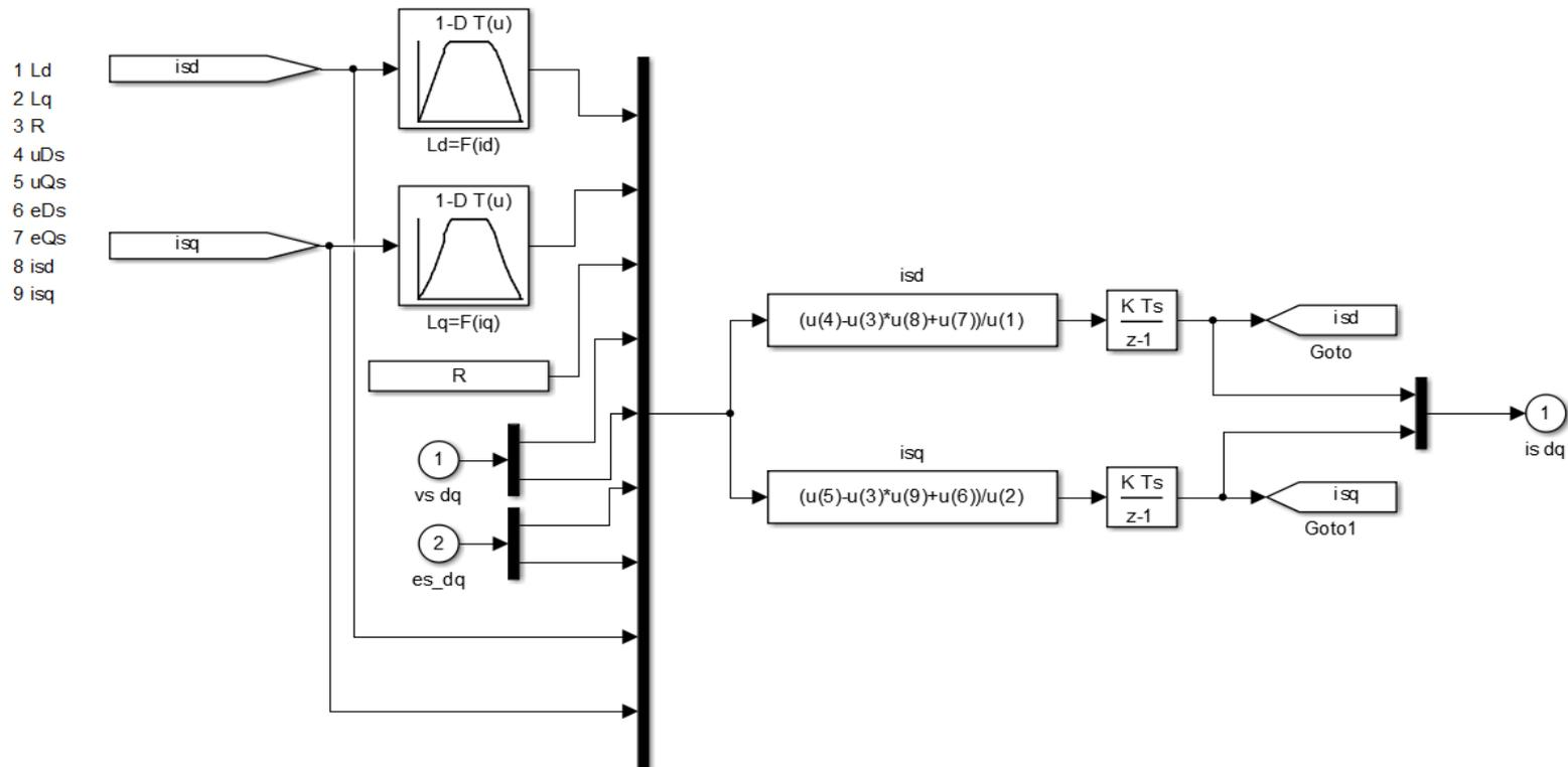
🐼  $R_s=0.2$  [ $\Omega$ ];  $\Psi_{md}=0.1025$  [Wb];  $\Psi_{mqd}=0.00002673$  [Wb];  $J=0.0048$  [ $\text{kg}\cdot\text{m}^2$ ],
