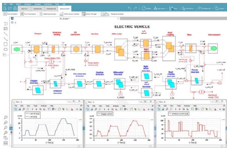
Fig. 7 EMR-based simulation of the Renault ZOE in AMESim
