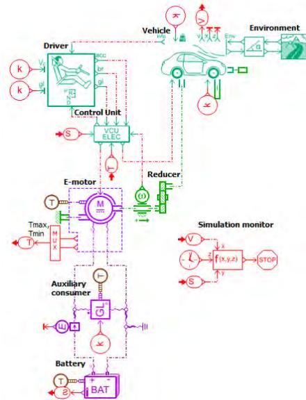
Figure 1: Sketch of a simple electric vehicle model - structural-based descriptions
