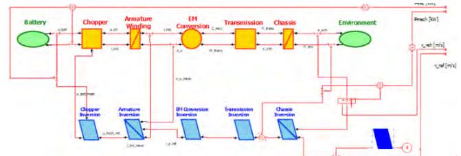
Figure 2: Sketch of an EMR functional-based electric vehicle model
