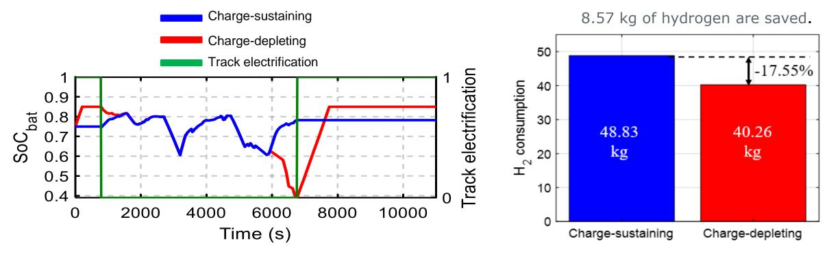
For this specific use case (track and sources sizing), the range can be increased by around 25km on this single track thanks to EMS.
